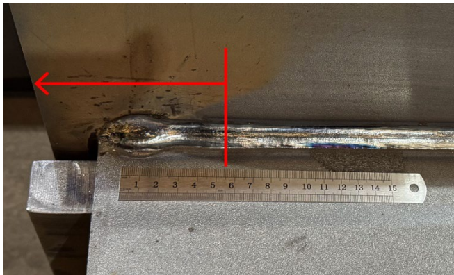
Figure 1. Start of weld characterised by large weld bead
