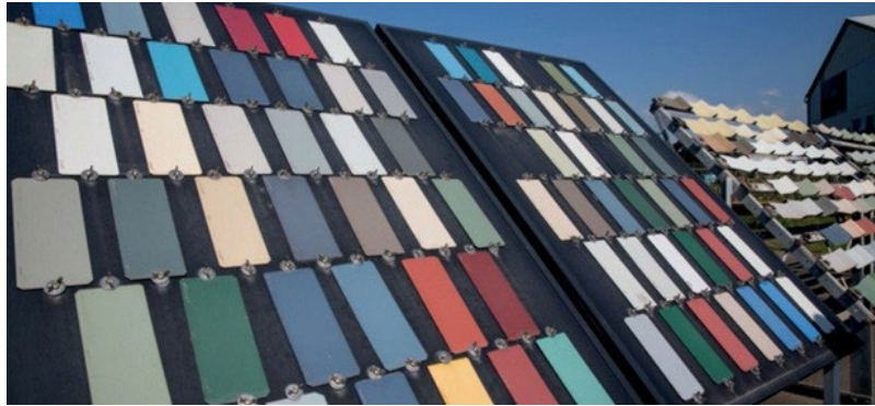
Figure 5. Outdoor exposure racks, located at various Australian sites, help BlueScope understand the Thermal Performance of its products over time.
