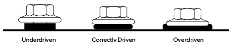
Figure 1. Correct tightening (driving) of fastener
