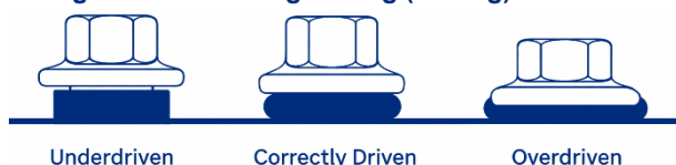
Figure 1. Correct tightening (driving) of fastener
