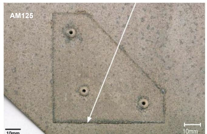
NOTE: The samples shown in Figure 3 have been tested in a severe environment to accelerate corrosion rates. Use of the product in this location is not recommended by BlueScope
