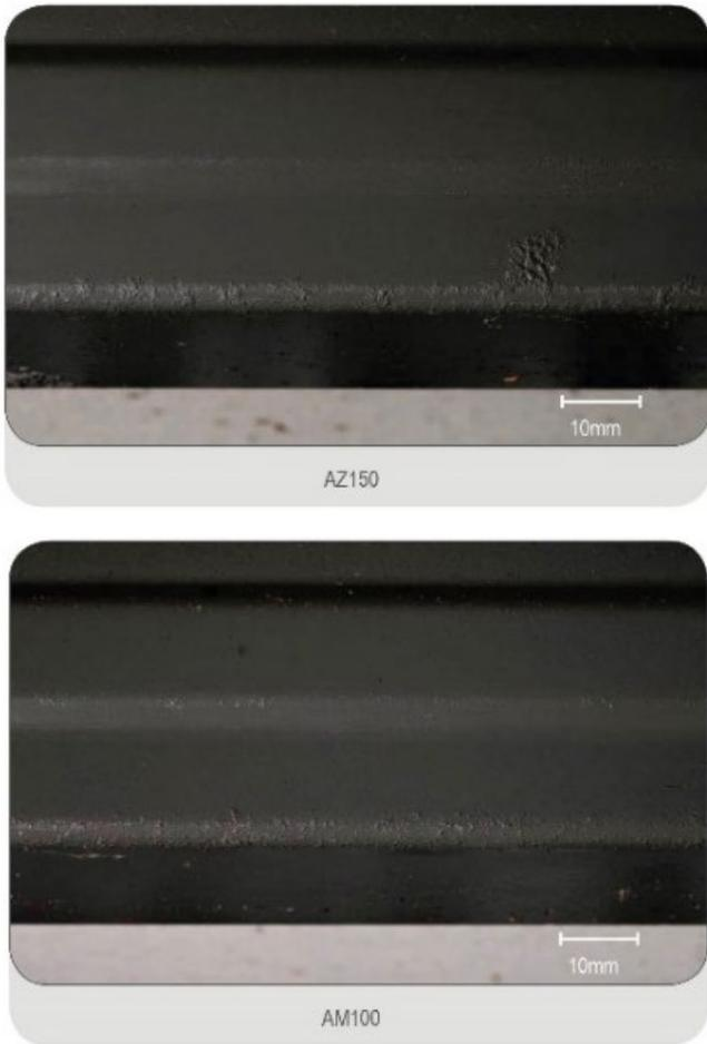
*NOTE: The samples shown in Figure 7 have been tested in a severe environment to accelerate corrosion rates. Use of the product in this location is not recommended by BlueScope*
