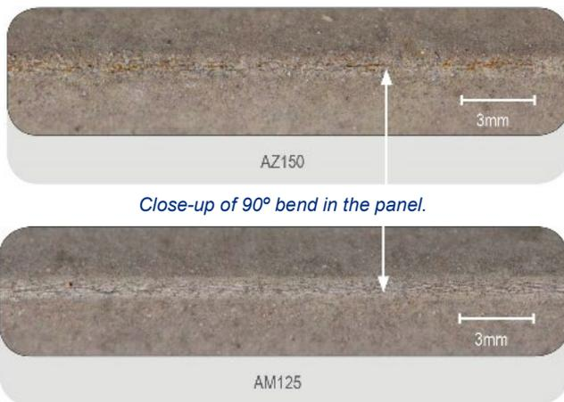
*NOTE: The samples shown in Figure 5 have been tested in a severe environment to accelerate corrosion rates. Use of the product in this location is not recommended by BlueScope.*
