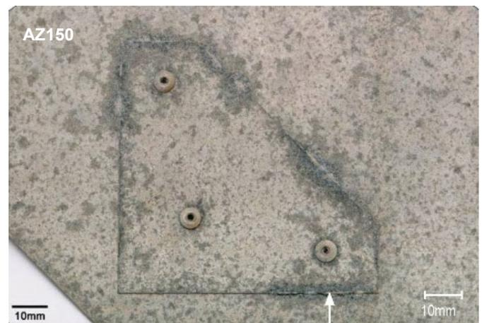
*Dark areas indicate metallic coating corrosion originating from the cut-edge.*
