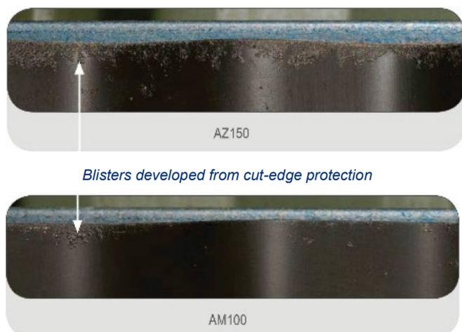
NOTE: The samples shown in Figure 4 have been tested in a severe environment to accelerate corrosion rates. Use of the product in this location is not recommended by BlueScope
