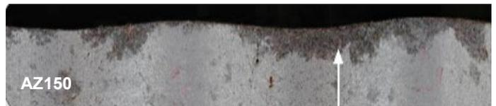
*Dark areas indicate metallic coating corrosion originating from the cut-edge.*
