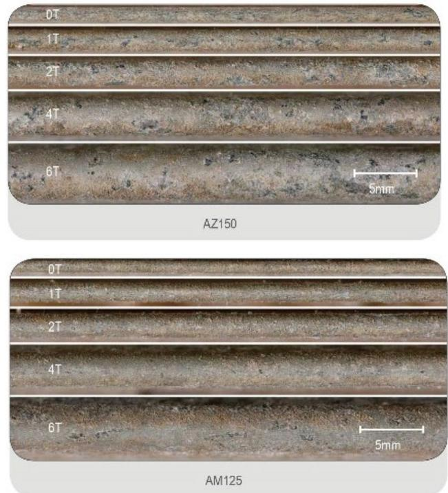
*NOTE: The samples shown in Figure 6 have been tested in a severe environment to accelerate corrosion rates. Use of the product in this location is not recommended by BlueScope.*
