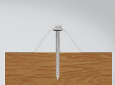
12 x 65mm Type 17 hex head screw or M6 x 65mm TS self drilling screw
