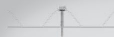
12 x 45mm Self drilling and tapping screw or M6 x 50mm TS self drilling screw (For 0.55mm thick battens use M6 x 50 TS self drilling screws)
