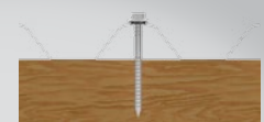
12 x 65mm Type 17 hex head screw or M6 x 65mm TS self drilling screw
