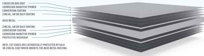
FIGURE 1.0 - STRATCO STEEL CROSS SECTION
