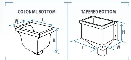
Specify the length, width and height when placing an order.
