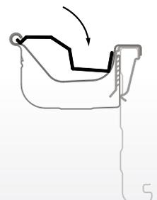
**TECHNICAL INFORMATION:** *Torrent Spacer Gutter Clip - Minimum allocated gap tested to stated overflow capacity. Gutter Slots - Minimum slot set-down tested to beyond stated overflow capacity. All testing performed at Stratco Testing Facility, Gepps Cross, South Australia.*
