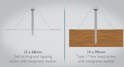
If fixing over an insulation blanket the next standard screw length to that indicated may be required with minimum 25mm timber embedment to be maintained.
