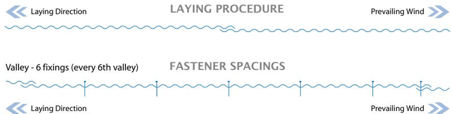
Side lap fixing is recommended at mid-span for support spacings that exceed 900mm.
