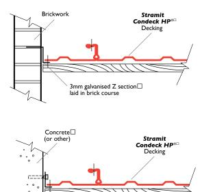
3mm galvanised □ angle bolted to wall□ at 900mm centres
