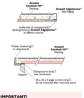
Edges of metal deck slabs exposed to direct or indirect rainfall must have a continuous drip feature to prevent water running to the underside of the
