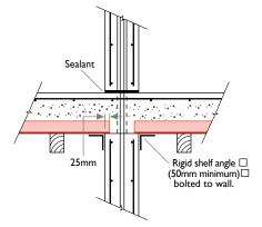
NOTES: 1. Standard end bearing of sectors. **Condeck HP**® Decking is 50mm. 2. For 25mm end bearing, end of sheets must be fastened to support.
