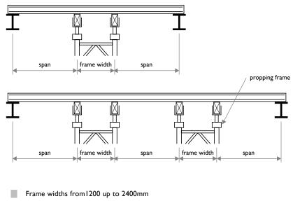
Frame widths from 1200 up to 1800mm
