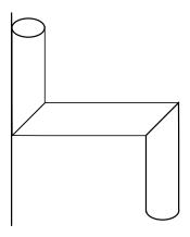
7. To extend downpipe to drainage level simply add extra lengths using the big and small end system.
