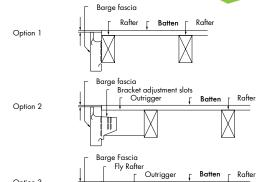
Cut both ends of the barge at an angle to suit the pitch of the roof. A Barge mitre is used to finish the joint between the barge and the Fascia. At the roof apex the 2 Barge lengths are joined by leaving a flange on one which inserts into the other and is secured by blind rivets.
