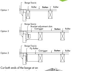
angle to suit the pitch of the roof. A Barge mitre is used to finish the joint between the barge and the Fascia. At the roof apex the 2 Barge lengths are joined by leaving a flange on one which inserts into the other and is secured by blind rivets.
