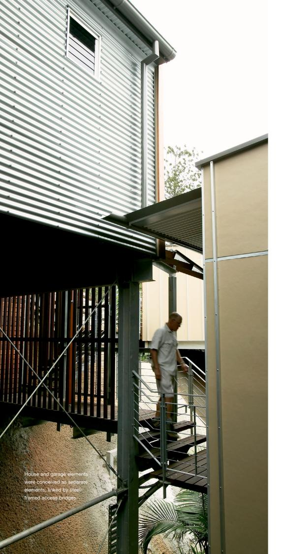
Also in response to the difficult site, the construction method employed lightweight steel, hardwood and LVL elements, with timber cladding internally and externally, and a range of steel elements throughout.
