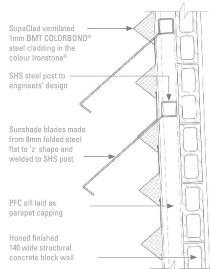
SupaClad ventilated 1mm BMT COLORBOND® steel cladding in the colour Ironstone®
