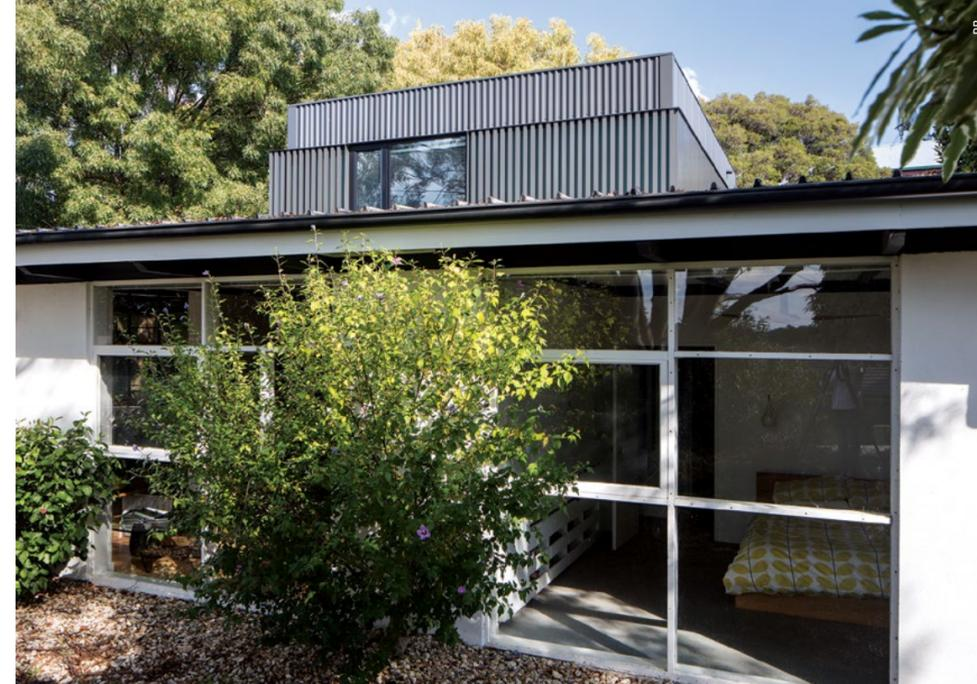
OPPOSITE: The dark-coloured cladding made from COLORBOND® steel in Stramit Longspan® profile, in the colour Nightsky® contrasts with the light-coloured roofing – which is done in COLORBOND® Coolmax® steel in Stramit Speed Deck® 500 profile, in the colour Whitehaven® – forming an effective heat barrier
