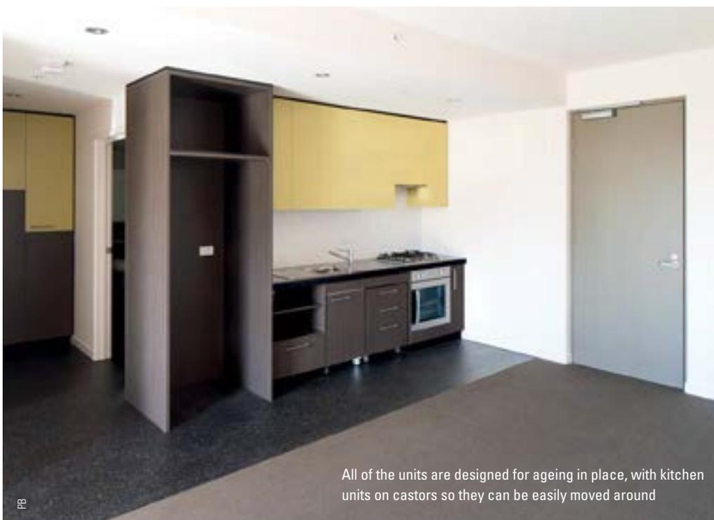
All of the units are designed for ageing in place, with kitchen units on castors so they can be easily moved around
