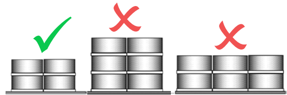
Two abreast, two high maximum! Stacks above this are NOT suitable using this guideline and require special restraint methods.
