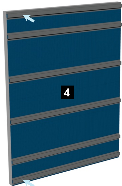
4 Install auxiliary tophats for flashings support on top and bottom of wall.
