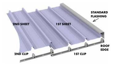
3. Fix the clip as indicated. Ensure the clip is 90° to the edge of the sheet and facing the direction required for laying.
