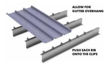
10. The order in which the ribs are snapped into place is important. Start with Rib 2, then the adjacent Rib 3 and move to the next purlin and repeat.
