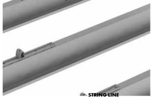
5. In accordance with the manufacturers recommendations, fix the Hex-head fasteners through the top of the clip into the support member.
