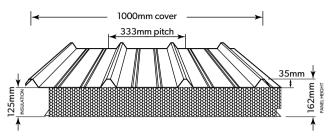
PERMALITE ALSULATE-125<sup>®</sup> insulated sandwich panel system is a roofing system with both insulative and structural advantages. The clever sandwich design incorporates both roofing and a prefinished ceiling using 5251 H38 Marine grade aluminium to provide outstanding watertightness, durability and stunning aesthetics. A variety of flashings and ridge covers cap off the roof design.
