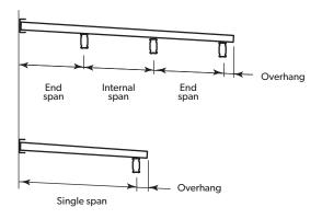
Note: For double spans use the end spans.
