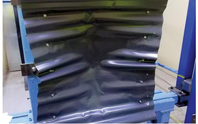
Typical debris impact test photographs
