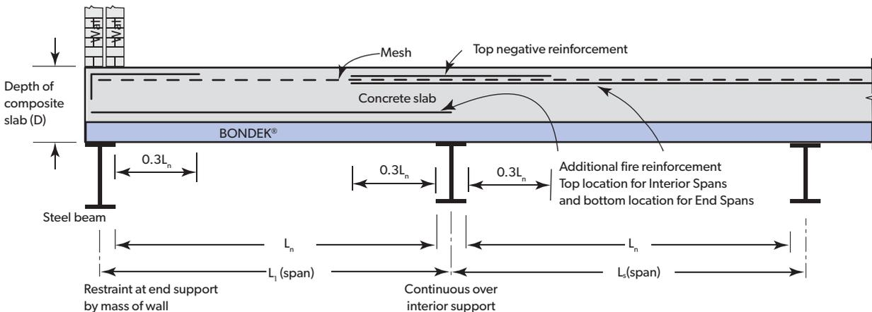
Note: 1/3 top negative reinforcement shall continue all over the span if ratio of live load to total dead load is more than 2.
