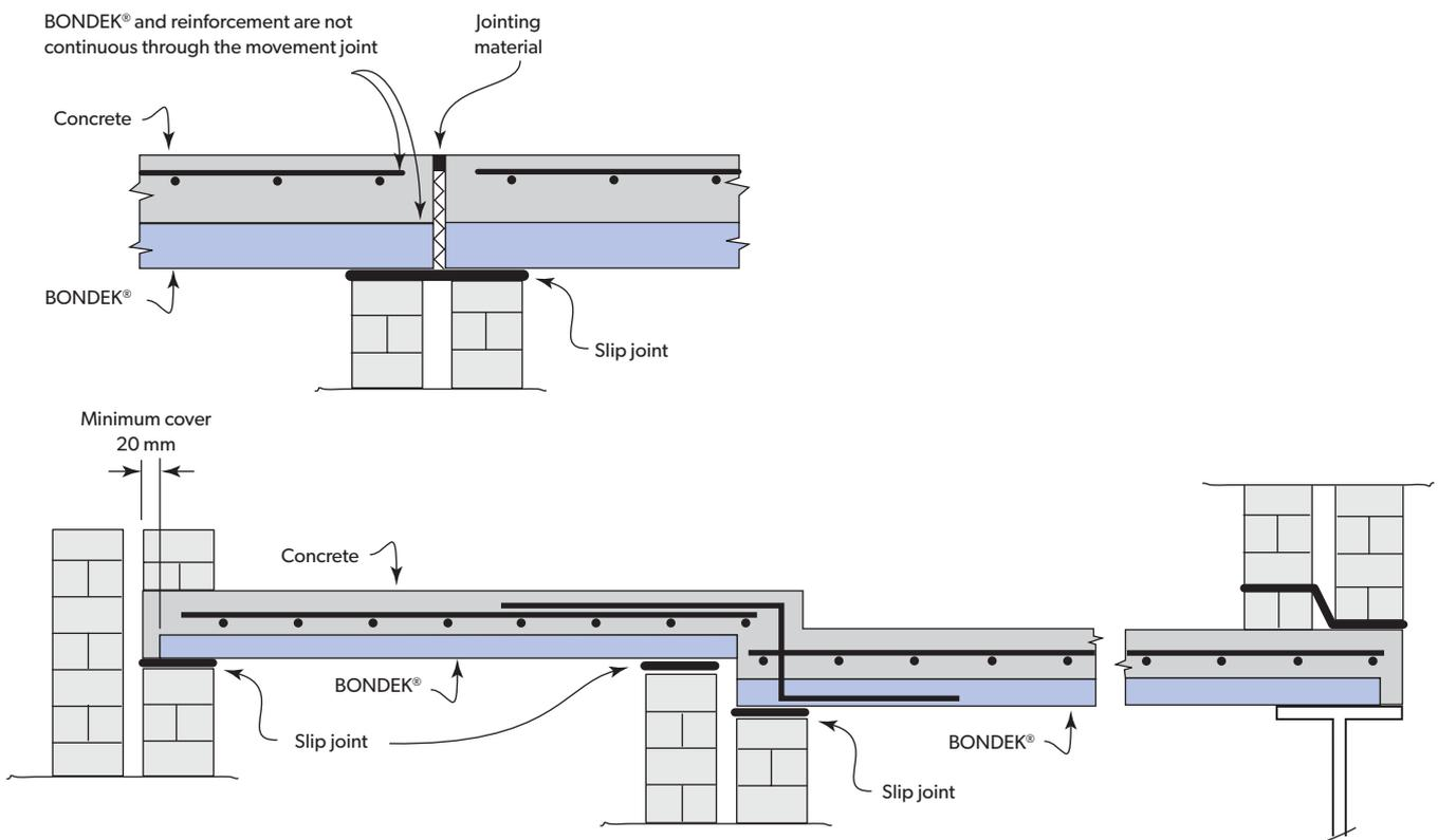
To prevent the cracking, BONDEK® slabs are not usually installed directly on brick supports, although this is not always the case in earthquake construction.
