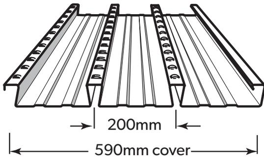
BONDEK® is a highly efficient, versatile and robust formwork, reinforcement and ceiling system for concrete slabs. It is a profile steel sheeting widely accepted by the building and construction industry to offer efficiency and speed of construction.
