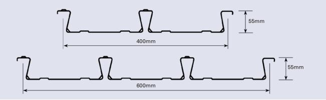
Fielders RF55<sup>®</sup> is a traditional flat pan or 're-entrant' profile that provides unmatched performance in suspended concrete slabs. RF55<sup>®</sup> is used in both concrete and steel frame construction and utilises patented technology to achieve superior spanning capabilities, less deflection and greater composite strength than similar re-entrant profiles. RF55<sup>®</sup> comes complete with a range of accessories allowing for easy suspension of ceilings and services.
