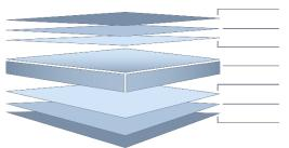
Finish Coat (Finish Coat + Primer = nominal 15µm) {Refer Notes 1, 3 & 4} Universal Corrosion Inhibitive Primer Conversion Coating Aluminium / Zinc / Magnesium alloy-coated steel with Activate<sup>®</sup> technology substrate Conversion Coating Universal Corrosion Inhibitive Primer Backing Coat (Backing Coat + Primer = nominal 10µm total) {Refer Note 5}
