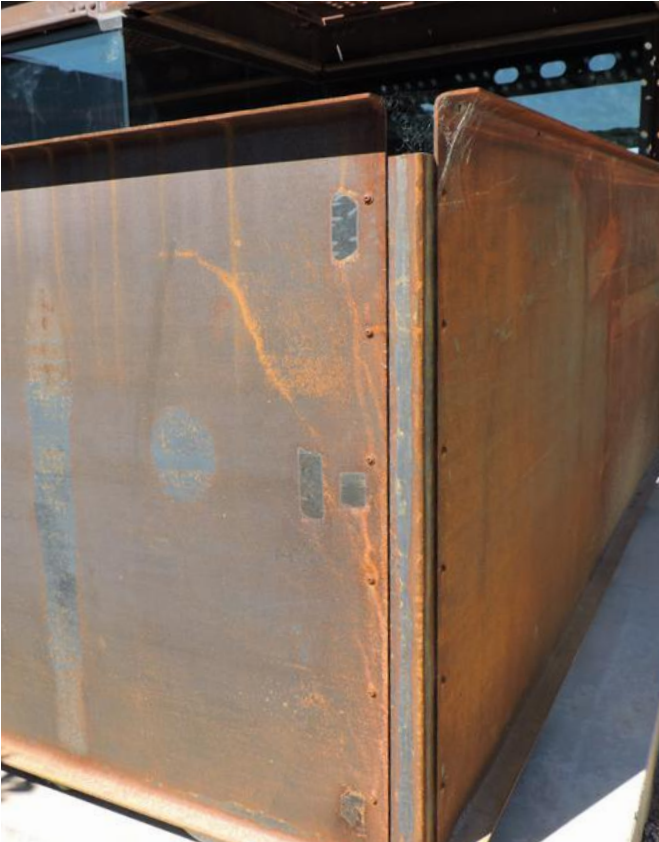
Figure 4-1: Example of surface contamination in the form of mill scale (above) and blasting of the steel surface (below)
