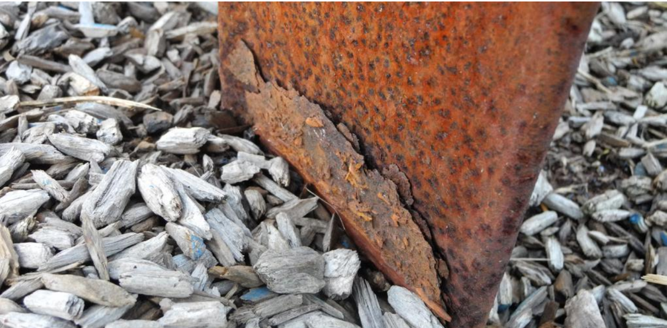
Figure 3-27: Example of ring bark corrosion on weathering steel sculpture, embedded in the ground
