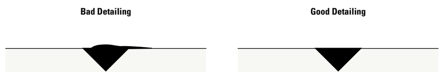
Figure 3.1 Grinding flush of welds which otherwise form water traps
