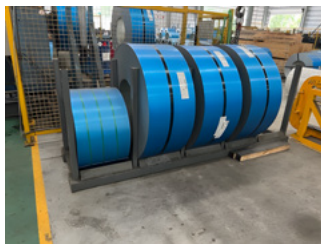
Figure 2. A rack used for separating narrow coil.
