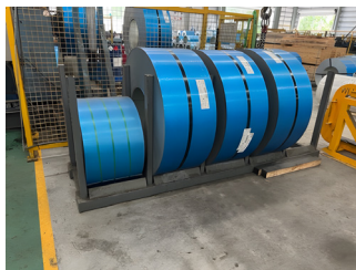
Figure 2. A rack used for separating narrow coil.
