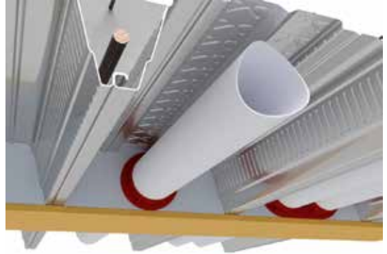
Penetration in ASB with fire collars installed
