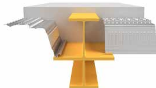
SlimDek 210® supported on UB with welded support plates
