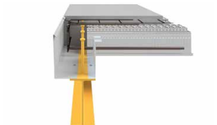
Downstand beam edge detail with SlimDek 210® perpendicular to beam
