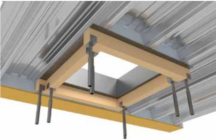
Large penetrations cutting maximum 1 x SlimDek 210® ribs - propping view
