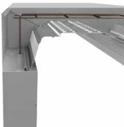
SlimDek 210® parallel to wall full sheet with edge form
