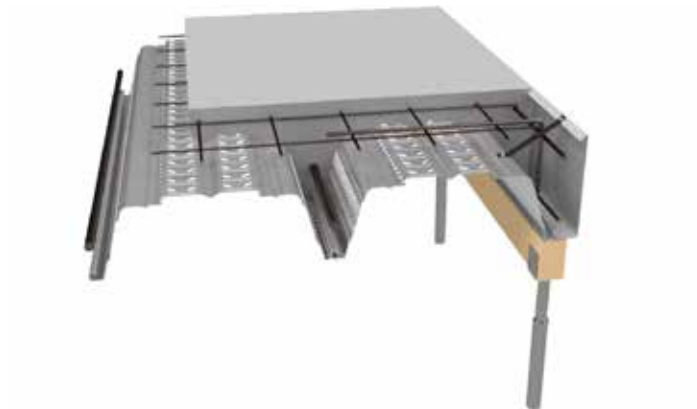
Unsupported edge detail full sheet with edge form - propping required
