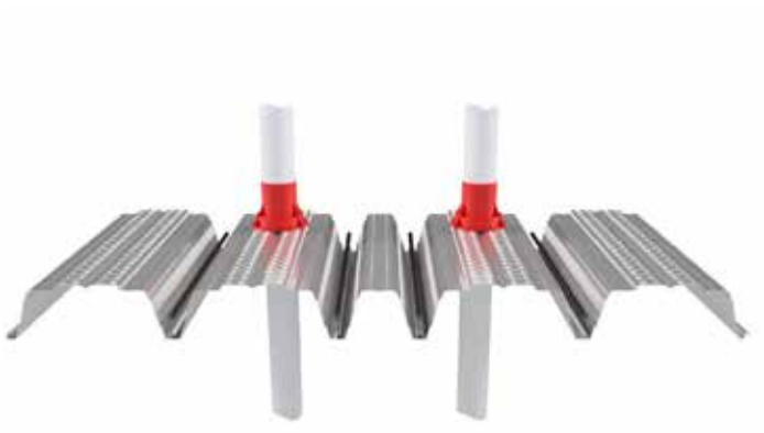
Max 400mm x 1000mm small penetrations not cutting SlimDek 210® ribs with timber form breakout
