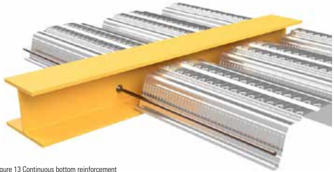
Figure 13 Continuous bottom reinforcement
