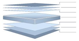
Finish Coat (Finish Coat + Primer = nominal 25µm) {Refer Notes 3 & 4} Universal Corrosion Inhibitive Primer Conversion Coating Aluminium / Zinc / Magnesium alloy-coated steel with Activate<sup>®</sup> technology substrate (can be zinc-coated) Conversion Coating Universal Corrosion Inhibitive Primer Backing Coat (Backing Coat + Primer = nominal 10µm total) {Refer Note 5}
