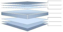
Finish Coat (Finish Coat + Primer = nominal 17µm) {Refer Notes 4 & 5} Universal Corrosion Inhibitive Primer Conversion Coating Aluminium / Zinc / Magnesium alloy-coated steel with Activate<sup>®</sup> technology substrate Conversion Coating Universal Corrosion Inhibitive Primer - for some foam backers or if specifically ordered Backing Coat (nominal 5µm total) {Refer Note 6}
