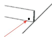
Rivet all sheet ends together 25mm from the end and 10mm above the pan using a 4.8mm dia 12.7mm grip aluminium blind rivet, through both underlap and overlap.
