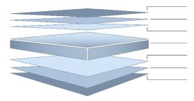
Finish Coat (Finish Coat + Primer = nominal 25µm) {Refer Notes 4 & 5} Universal Corrosion Inhibitive Primer Conversion Coating Aluminium / Zinc / Magnesium alloy-coated steel with Activate<sup>®</sup> technology substrate Conversion Coating Universal Corrosion Inhibitive Primer Backing Coat (Backing Coat + Primer = nominal 10µm total) {Refer Note 6}
