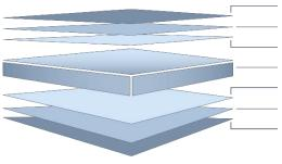
Finish Coat (Finish Coat + Primer = nominal 33µm) {Refer Notes 1, 5 & 6} Universal Corrosion Inhibitive Primer
