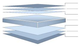
Finish Coat (Finish Coat + Primer = nominal 25 $\mu$ m) {Refer Notes 3 & 4} Universal Corrosion Inhibitive Primer
