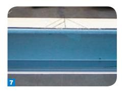
Mark the mitre lines on each of the flanges. And then mark a 12mm lap line on each flange.
