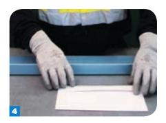
Place it on the bench, and fold it flat to get a definite fold in the cardboard. Then, place the cardboard back on to the stud section and form the second corner.
