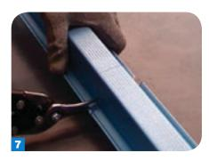
To cut roof battens, cut in at an angle on the lip to free up the lip material.
