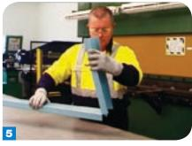
Once both flanges have been cut, bend the piece back and forth until the section snaps apart.
