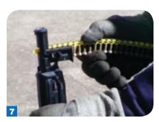
Collated screw magazines are easily inserted or removed into the 'Quik-Drive Pro' tool.
