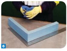
Bend the steel into a 90° angle checking the angle with your square.
