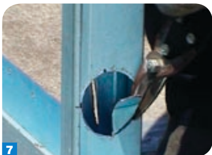
7 Finally, use your left and right snips to cut out the circles from the top down.
