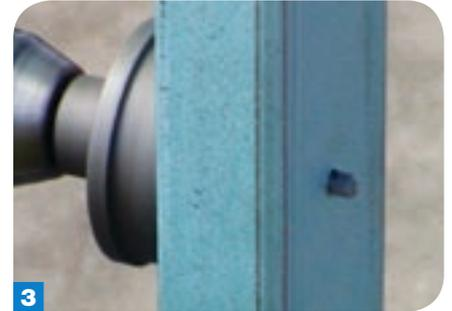
**3** Once the first side is penetrated, push through to locate the pilot hole on the other side.
