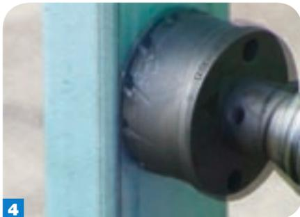
**4** Using the pilot hole, drill back from the other side to complete the hole.
