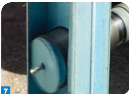
**7** Then drill until both wall thicknesses are penetrated.
