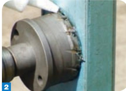
**2** Use a lubricant to assist with cutting and extend the life of the cutter.
