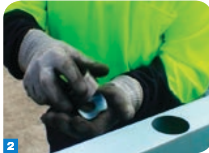
2 Remove the slug by slipping off the chuck.
