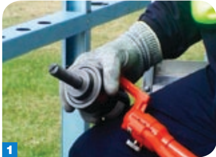
1 A hydraulic punch has a fast action slip on/off chuck making it quick and easy to use.
