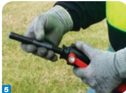
5 Larger penetration holes are achieved by fitting a larger mandle into the tool.
