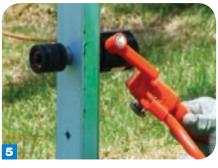
When multiple holes are required, save time by making all your pilot holes first, and then follow up with a hydraulic punch.
