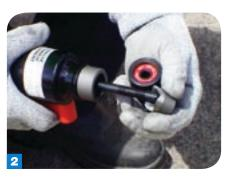
Hydraulic punches can be used to make holes in a range of steel thicknesses.
