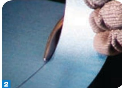
**2** Both left (red) and right (green) snips allow you to cut in a straight line. Mark your line with a marker and ruler before cutting.
