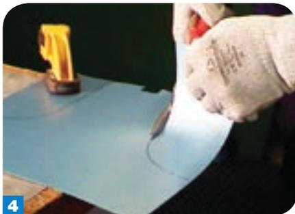
**4** When cutting with snips, make sure the scrap is peeled away. This will make it easier on the blades and will make it easier for you to accurately guide the snips.
