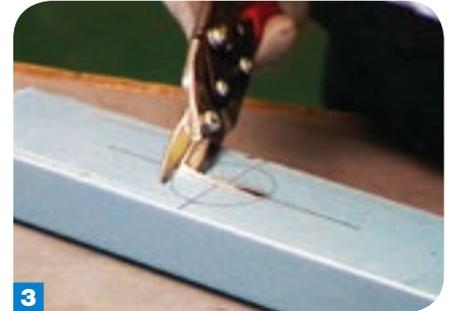
**3** Left cut snips (red) allow you to cut in a curved direction to the left. Right cut snips (green) allow you to cut in a curved direction to the right.
