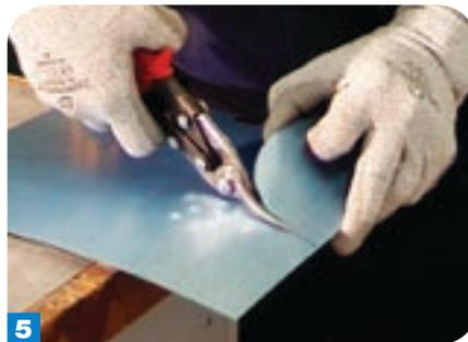
**5** When cutting, don't take large bites. Cut with small cuts (approximately 5–10mm) moving the blades forward to create a neat and continuous cut.
