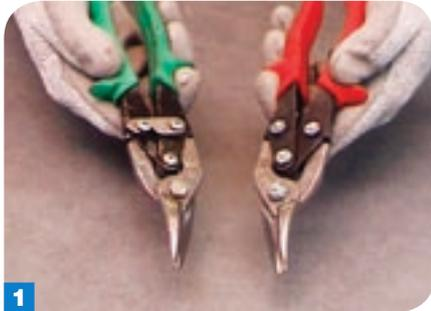
**1** We recommend using left-offset and right-offset aviation snips. The term 'offset' refers to the blade being offset to the handle – allowing you to work above the material being cut. The red handled snip is the left cut snip. The green handled snip is the right cut snip.
